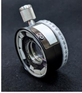
Figure 1: Modified Stokes lens
