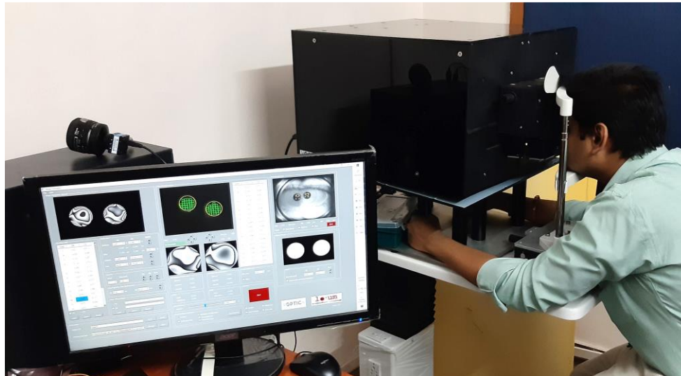
Figure 2: First prototype of the proposed Binocular VAO with control software
